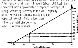
Pounds of vapor left in a 350 Ton chiller at various vacuum levels
