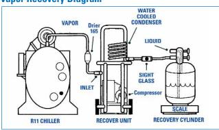
Once all the liquid has been recovered, the remaining vapor can be extracted with the recovery unit as shown in the diagram above.
