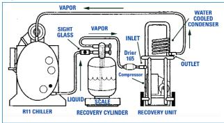
Liquid recovery is done by using the push-pull method as shown in the diagram above. A lower pressure is created in the recovery cylinder which forces the liquid refrigerant from the chiller into the cylinder.
