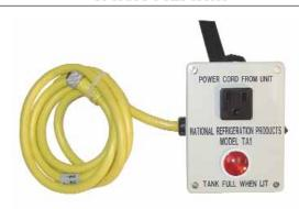
Provides positive shut-off for recovery units without tank overfill protection. With power cord-to-tank adapters (see below), the TA1 can be used on any tank utilizing a float. The TA1 comes with 5 feet of float cord and a velcro strap for easy mounting.
