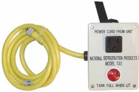
Provides positive shut-off for recovery units without tank overflow protection. With power cord-to-tank adapters (see below), the TA1 can be used on any tank utilizing a float. The TA1 comes with 5 feet of float cord and a velcro strap for easy mounting.
