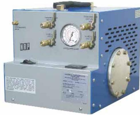
The RAD700 is a recycling unit to be used on the job site in conjunction with a LV2000, LV1, ULV1, LV1C, LV1CUL, GS1, GS1UL, GS2, REVAC, and AR1UL or other recovery units. It is designed to recycle refrigerant in batches of 40lbs., to a quality within the IRG2 standard. The RAD700 has been tested in accordance to the ARI-740 standard.
