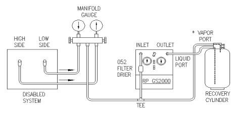
\* OPEN VAPOR PORT ON TANK WHENEVER TANK PRESSURE EXCEEDS 350 psi.
